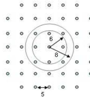
**Figure 8.** The simulated network topology is a square grid. The distance between neighbouring nodes is 5 units. The number of neighbours a node has depends on its transmission radius.
