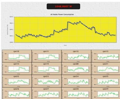
Fig. 2. Power monitor visualizer web view.
