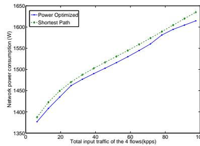
**Fig. 4** Power consumption for proposed algorithm compared to shortest path with four flows and power optimisation
