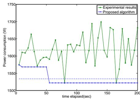
**Fig. 6** Power consumption for proposed algorithm with memory
