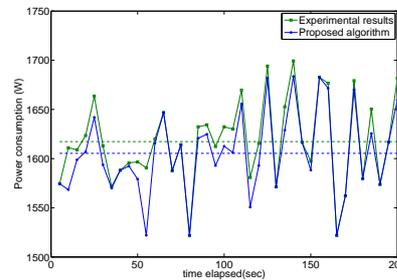
**Fig. 5** Power consumption for the gradient algorithm (green) compared to power-based EARP [4]
