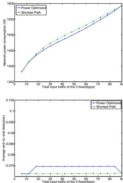
**Fig. 3** Power consumption (above) and end-to-end delay with power and delay optimisation (below)
