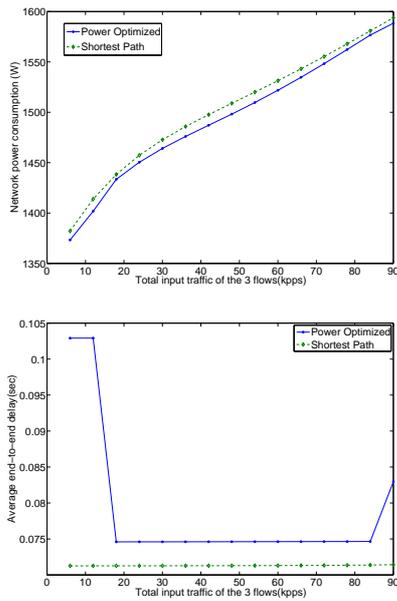
**Fig. 2** Power consumption (top) and average end-to-end packet delay (bottom) against varying traffic load in Kpps (kilo-packets per second) for power-optimised versus shortest path routing
