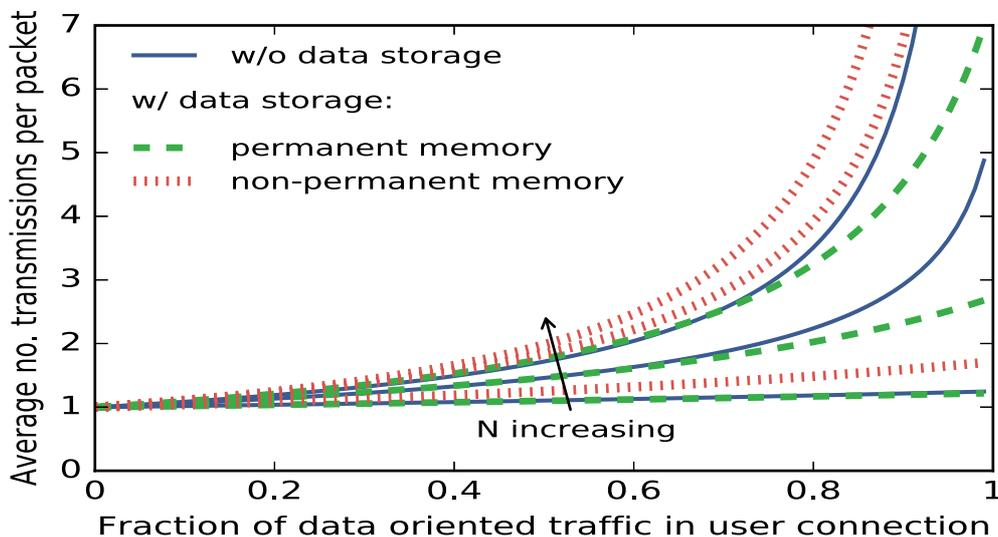
**Fig. 2.** Average number of transmissions per DP versus the fraction  $p$  of DPs that must be retransmitted if lost. The length of the path traversed by user traffic is set to  $N = 1, 5, 10$  hops. Other parameters are  $\lambda = 0.1$  DP/sec,  $\Lambda = 0.9$  DP/sec,  $\gamma = 0.9$  EP/sec,  $\delta = 0.1$  EP/sec, and the service rate of the DPs is  $\mu = 0.9$  DP/s.
