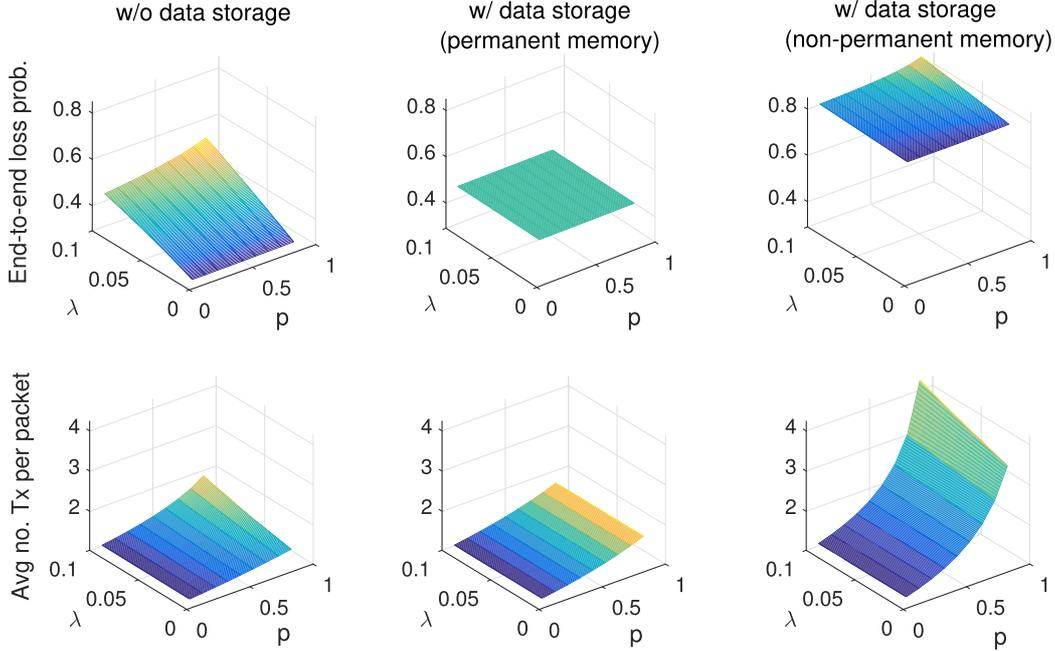
**Fig. 3.** The end-to-end loss probability (top) and average number of transmissions per DP (bottom) against the DP rate  $\lambda$  and the fraction  $p$  of DPs that must be retransmitted if lost. The number of hops in the path traversed by the user traffic is fixed at  $N = 3$ , while the other parameters are as in Fig. 2.
