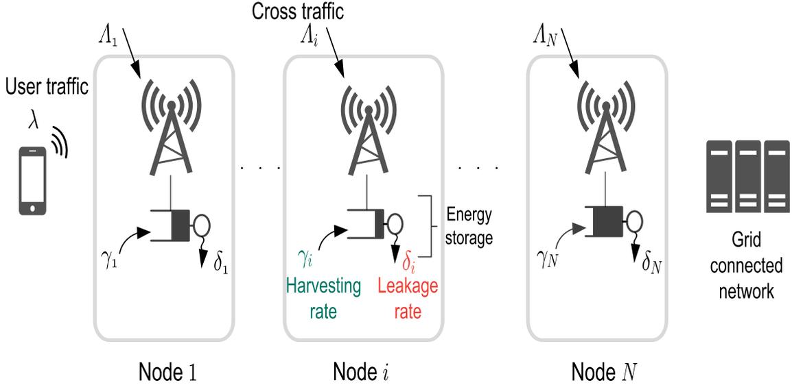
**Fig. 1.** Schematic representation of a multi-hop mobile access network with intermittent energy.
