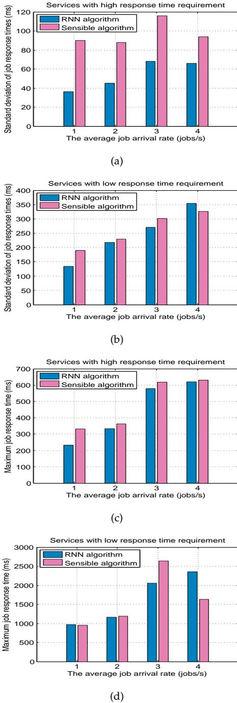
Fig. 13. The standard deviation of the measured response time, and its maximum value as a function of the task arrival rate ( $x$ -axis), for the two classes of tasks when task allocation uses the Goal function including both the economic cost and the penalty (11). Note that the performance of the RNN and Reinforcement Learning based algorithm, and the Sensible Algorithm are being compared.
