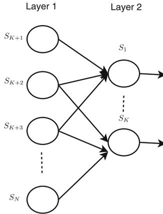
**Fig. 2.** A network of EHWSs with two layers. In this case packets are forwarded by at most one node.
