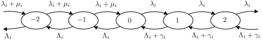
**Fig. 1.** CTMC underlying the model of sensor  $i$
