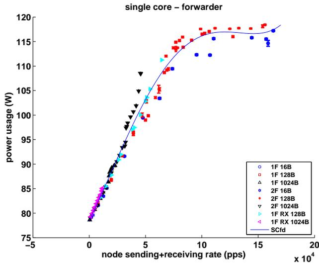
Figure 1: Power consumption as a function of packet rate for a single core router [12]
