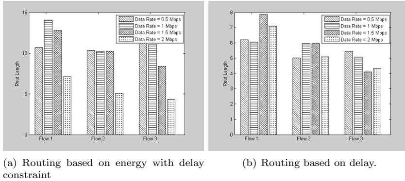
Figure 4: Average length of the end-to-end path taken by the three active flows.
