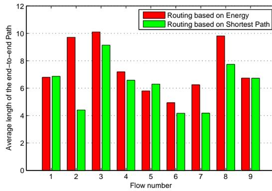
Figure 11: Scenario two: Average length of the end-to-end path taken by each of the nine active flows.
