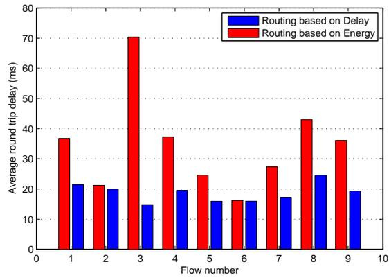
Figure 10: Scenario two: Average round trip delay for each of the nine active flows in their lifetime.
