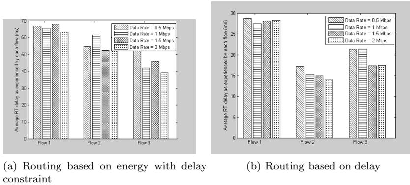
Figure 3: Average round trip delay for the three flows with different traffic levels
