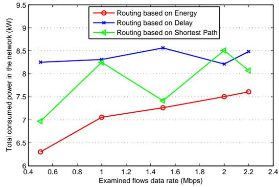
Figure 9: Scenario two: Total power consumption in the network vs. traffic rate of the examined flows
