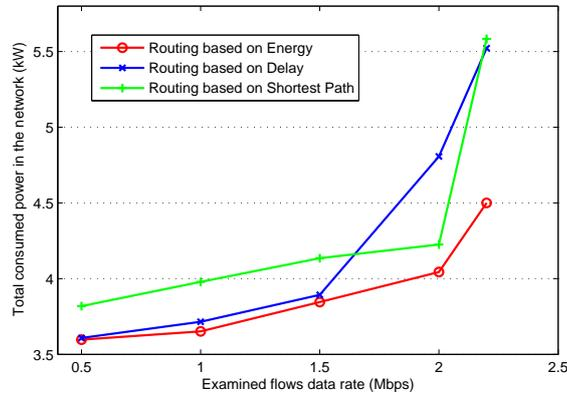
Figure 5: Experiment with three flows: total power consumption in the network vs. traffic rate all connections.
